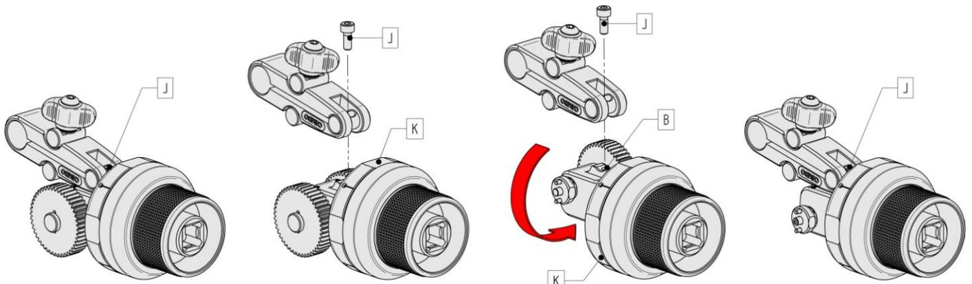
**Changing the rotation direction** (note: CW = clockwise and CCW = counter clockwise)
